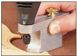
Dremel makes a little plastic router head that works well. Craftsman (Sears) makes a similar one shown here. I modify the basic design so the openings are large and drill a hole, glue in a fitting, and pump air at the cutting tip with an aquarium pump to clear away dust. Both Dremel and Craftsman can be found at many woodworking stores, Sears, and online from Widget Supply at <a href="https://www.widgetsupply.com">www.widgetsupply.com</a>.
