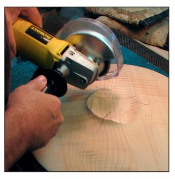
Step 2 - Remove material between the feet using a power carver. Here an Arbortech tool is used. Make the recesses rounded.
