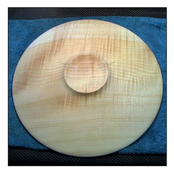
Step 1 - Turn a ridge from the tenon that has the cross-section of the foot you want to create. Mark where the three feet will go.
