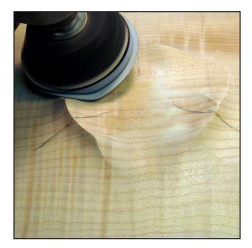
Step 3 - Use a power sander to smooth the areas between the feet. Change the angle of the sanding pad between the pads to make a uniform surface.
