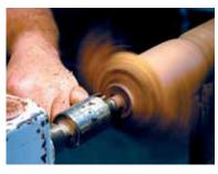
Step 16. Turn a recessed area in the foot. Take great care to avoid any contact between fingers and the rough-edged rapidly spinning pod.
