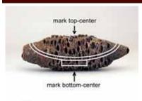
Step 1. Spend a few minutes determining how the banksia pod should best be positioned on the lathe. The outer tips should be solid (no seed holes). Mark the centerline for mounting.
