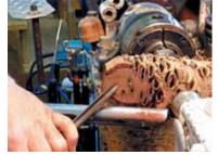
Step 3. Rough turn the bottom of the pod using a 1/2" bowl gouge. For a finishing cut, Dave prefers to use a pull-cut because he thinks that produces the cleanest cut. Do not use a scraper because it will tear the edges.
