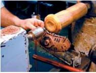
Step 14. Prepare to finish the foot by reversing the pod on the lathe. Dave uses a homemade support padded with leather to hold the work against the tailstock.
