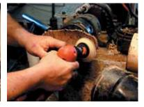
Step 12. Most mortals will need to start with a coarser grit, but Dave starts with 240. The lathe is off, and the sanding pad is positioned so its edge moves away from the pad
