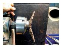
Step 10. Dave has finished turning the top side with the live center removed. Again use a sheet of blackened cardboard to check the form profile.
