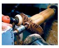
Step 17. Power sand the bottom side of the pod with the lathe off. Again, to prevent a sander catch, the sanding pad is positioned so its edge moves away from the pod during the process.
