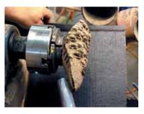
Step 7. After repositioning the work in his chuck, Dave checks that the "wings" on the pod are symmetrical by noting how far they extend along his tool rest.
