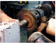
Step 8. Rough turn the top side of the pod, again using a 1/2" gouge. Stop frequently to check that the pod material does not have any flaws that will cause it to break on the lathe.
