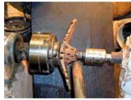
Step 9. The pod with the top rough turned about 1/4" thick. Keep the live center in place during all the roughing for better stability and safety.
