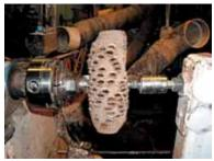
Step 2. Place the pod between centers on the lathe with the bottom towards the tailstock. Dave does not use a coneshaped live center in order to minimize damage to the pod's foot.
